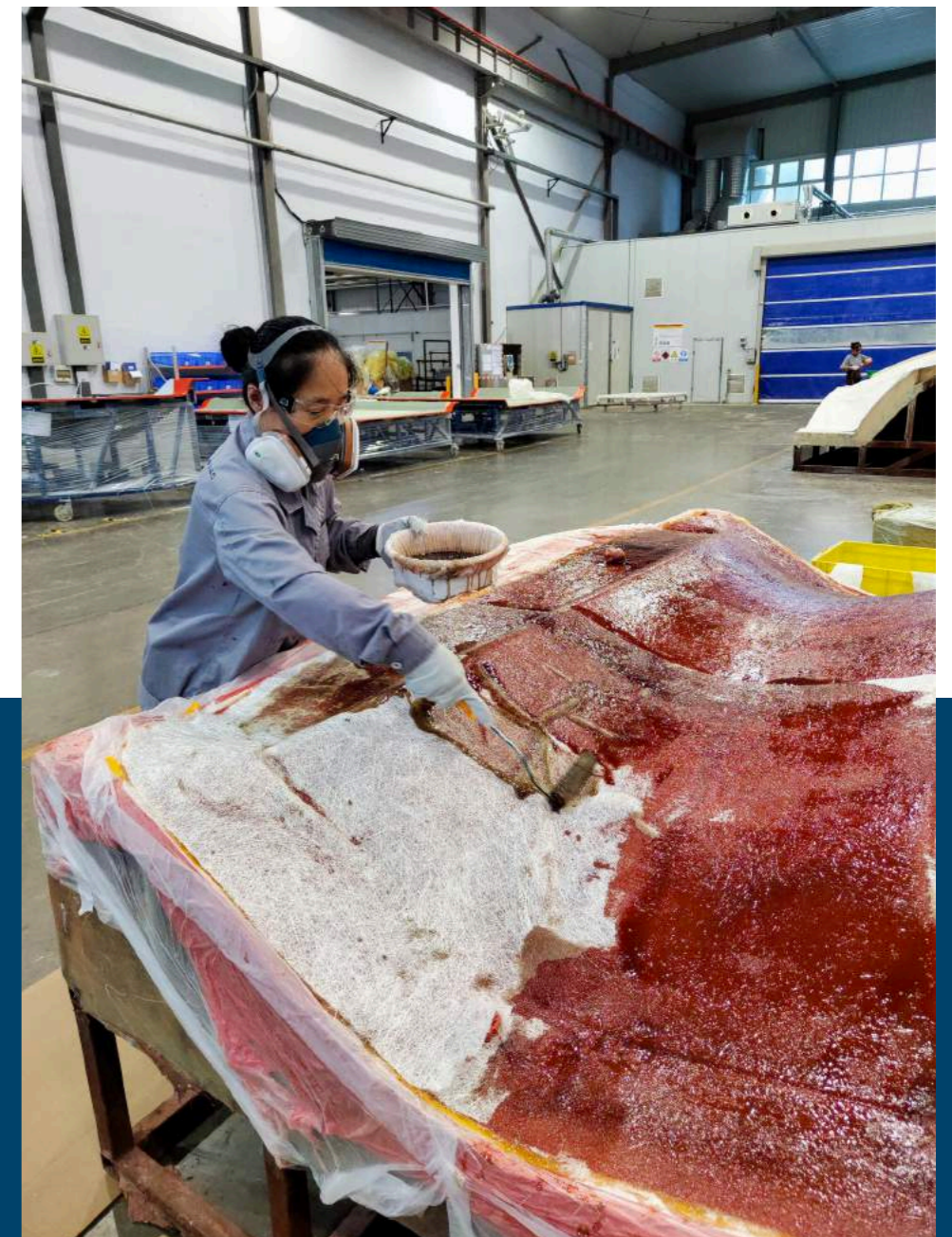
Photo: One of our employees repairing a fiberglass mould in our factory in China.
