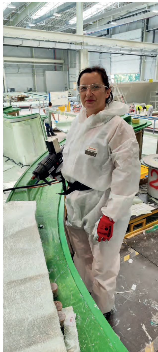
Operators using hot melt adhesive guns during the lamination process at our factory in Poland
